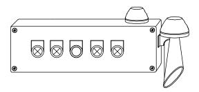
Example: Truck module with LEDs full/empty, key switch for control of the pinch valve, illuminated button for display and reset of alarm "silo full" and expulsion of the filing pipes, status LED for pinch valve
